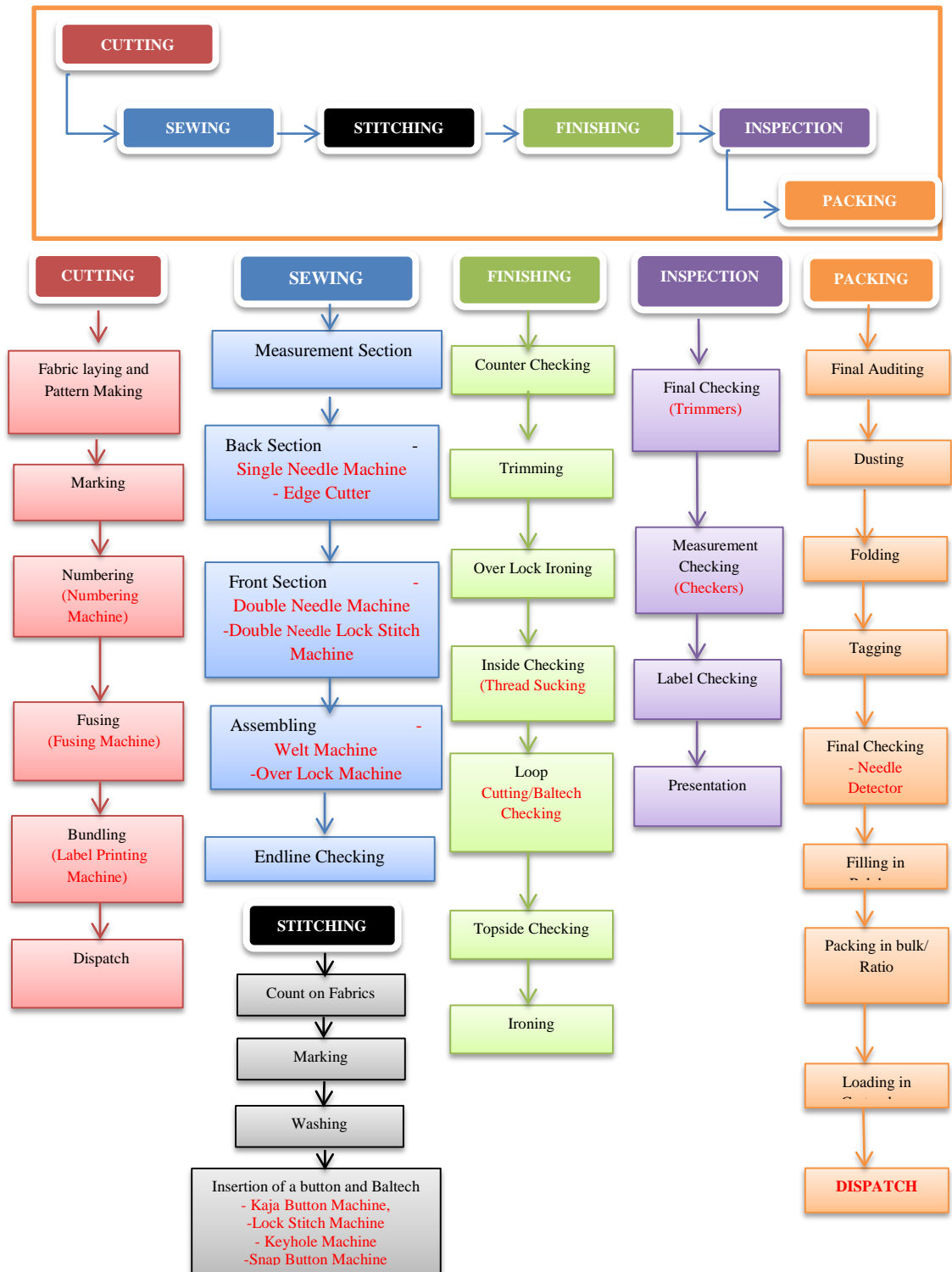
Figure 3.1: Process Flow of a Trouser manufacturing
